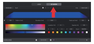
**7.** To add gradient stops to your pattern element, click the plus button under **SET LIGHTING**. Gradient stops will allow you to add multiple colors in one element. Click the gradient stop and add a new color to the designated area by clicking the desired color in the color palette. The more stops you add, the more colors you can add, but the shorter the colors will become.
